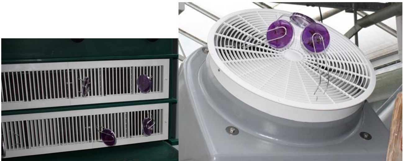
Picture 1. Air in (left) and air out (right). Petri dishes of 90 mm Petri dish arranged at 45° angle on the lid.
